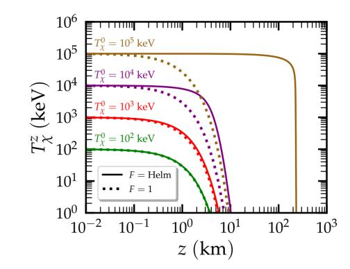
To further visualize the Earth attenuation and finite nuclear size effects, we demonstrate the DSNB-boosted DM flux for unattenuated and attenuated cases in the following diagram, assuming  $m_{\chi} = 300$  MeV, and  $\sigma_{\chi e} = \sigma_{\chi n} = 10^{-29}$  cm<sup>2</sup>.
