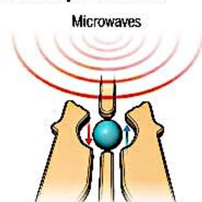
These “artificial atoms” are made by adding an electron to a small piece of pure silicon. Microwaves control the electron’s quantum state.
