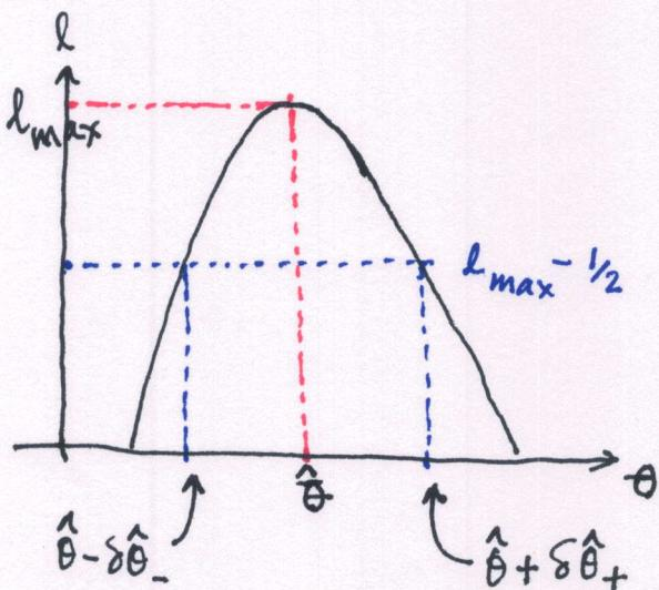
$$\begin{aligned} l(\hat{\theta} + \delta\hat{\theta}) &= l_{\max} + \frac{1}{2} \left( -\frac{1}{\hat{\sigma}_{\theta}} \right)^2 \cdot \delta\hat{\theta}^2 \\ &= l_{\max} - \frac{1}{2} \end{aligned}$$
